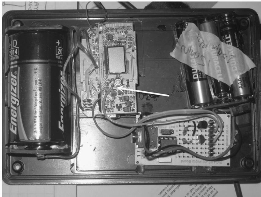
FIG. 2. Layout of VQ1005 camera unit. At left is alkaline D cell to power camera. Next is camera itself [case removed, so circuit boards are exposed, showing liquid crystal display (LCD) status display]. A wire to the mode switch terminal from the microcontroller board is arrowed. At lower right is the microcontroller board with switching transistors, and above that is the 3-AAA cell power for the microcontroller.
